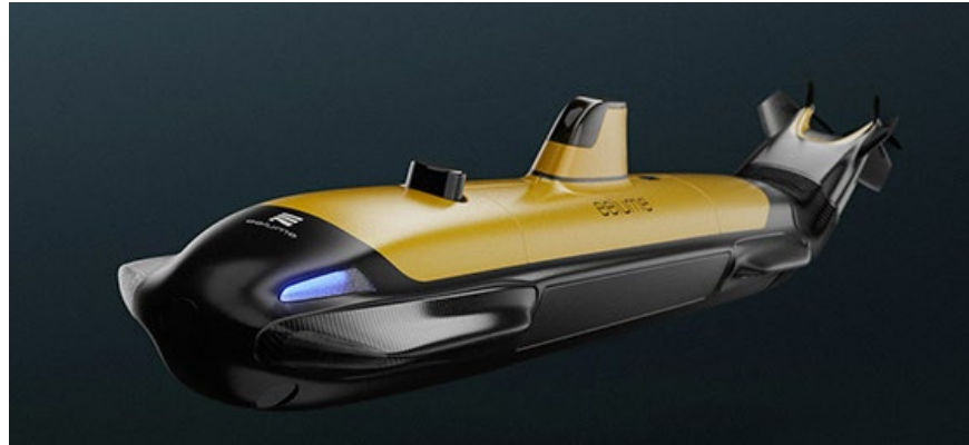
Figure 3. Eelume S Series All-Terrain AUV can come equipped with 4K still camera and MAS systems (Eelume, 2025).
